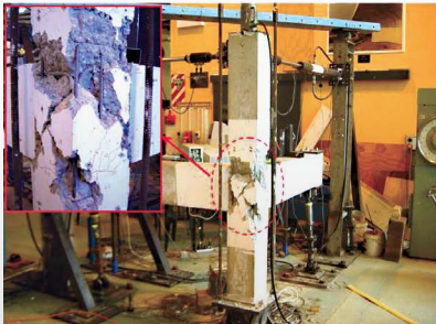
(b) Beam bars bent in - loss of joint integrity
